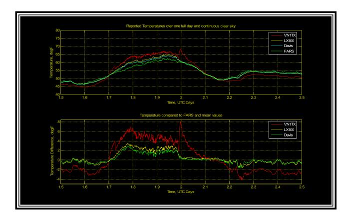
Most obvious in the VN1TX data are the "bat ears" at x-axis locations of about 1.73 and 2.0 where the aspirating fan turns off and on. Because morning sun is shaded by trees until about 10:30AM local time, the morning bat-ears are less pronounced -- when the
