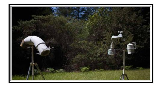
All sensors are wireless, with the exception of a DC fan power connection to the FARS.
